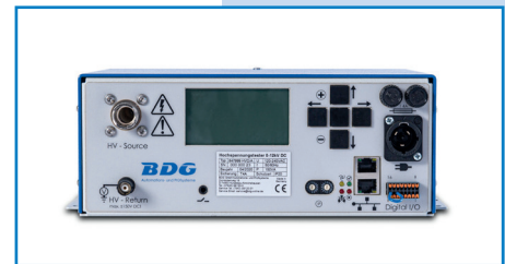
ElMeS™ as a high-voltage DC tester
