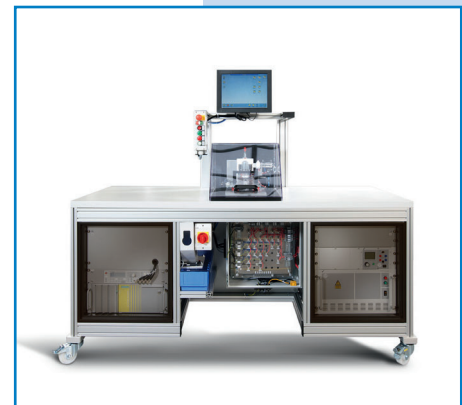
Universal test rig with built-in ElMeS™ high-voltage DC tester
